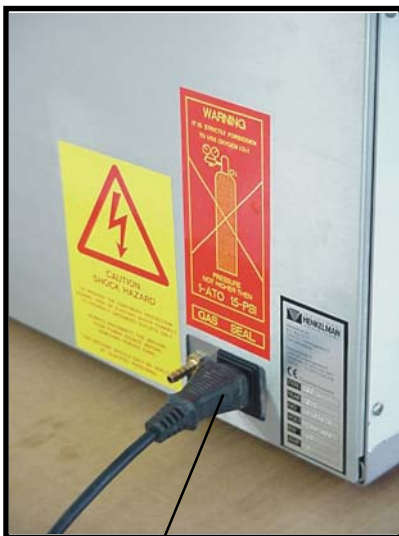
Main power supply
